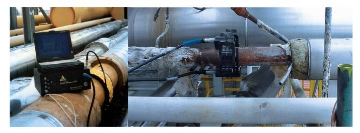
Fig. 3: Guided wave technology applied on pipe racks
