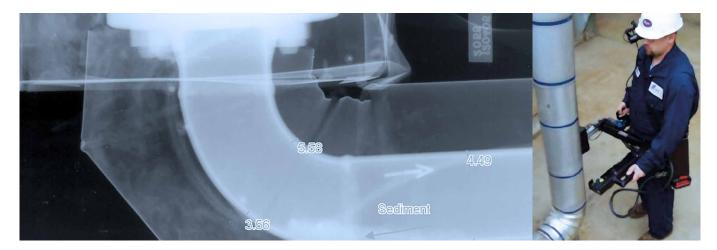
Fig 4: Digital radiography (right); Real time video profilometry (left)
