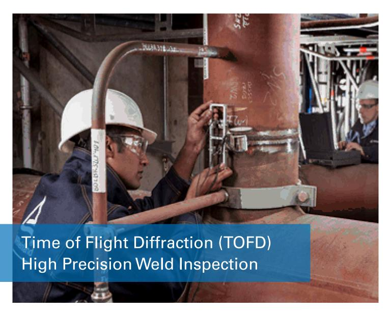
Fundamentals of an advanced non-destructive technique for reliable flaw detection.
